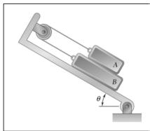
The 20-N block A and the 30-N block B are supported by an incline that is held in the position shown. Knowing that the coefficient of static friction is 0.15 between all surfaces of contact, determine the value of  $\theta$  for which motion is impending.
