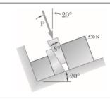
Two  $8^\circ$  wedges of negligible weight are used to move and position a 530-N block. Knowing that the coefficient of static friction is 0.40 at all surfaces of contact, determine the magnitude of the force **P** for which motion of the block is impending.
