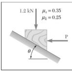
Determine whether the block shown is in equilibrium and find the magnitude and direction of the friction force when  $\theta$ = 25° and P = 750 N.
