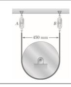
The setup shown is used to measure the output of a small turbine. When the flywheel is at rest, the reading of each spring scale is 70 N. If a 12.60 N·m couple must be applied to the flywheel to keep it rotating clockwise at a constant speed, determine (a) the reading of each scale at that time, (b) the coefficient of kinetic friction. Assume that the length of the belt does not change.
