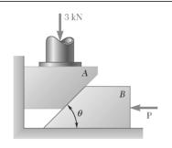
Block A supports a pipe column and rests as shown on wedge B. Knowing that the coefficient of static friction at all surfaces of contact is 0.25 and that  $\theta = 45^{\circ}$ , determine the smallest force **P** required to raise block A.
