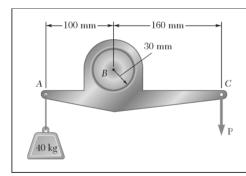
A lever of negligible weight is loosely fitted onto a 30-mm-radius fixed shaft as shown. Knowing that a force  $\bf P$  of magnitude 275 N will just start the lever rotating clockwise, determine (a) the coefficient of static friction between the shaft and the lever, (b) the smallest force  $\bf P$  for which the lever does not start rotating counterclockwise.
