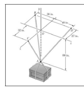
A crate is supported by three cables as shown. Determine the weight of the crate knowing that the tension in cable AB is 750 lb.
