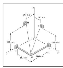
For the frame and cable of Problem 2.87, determine the components of the force exerted by the cable on the support at E.
