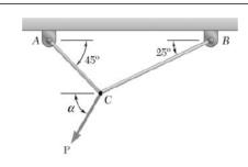
Two cables are tied together at C and are loaded as shown. Knowing that P = 500 N and  $\alpha = 60^{\circ}$ , determine the tension in (a) in cable AC, (b) in cable BC.
