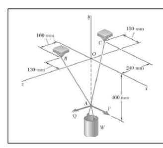
A container of weight W is suspended from ring A. Cable BAC passes through the ring and is attached to fixed supports at B and C. Two forces P = Pi and Q = Qk are applied to the ring to maintain the container in the position shown. Knowing that W = 376 N, determine P and Q. (Hint: The tension is the same in both portions of cable BAC.)
