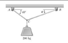
Two cables are tied together at C and are loaded as shown. Knowing that  $\alpha = 20^{\circ}$ , determine the tension (a) in cable AC, (b) in cable BC.
