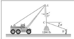
Knowing that  $\alpha = 20^{\circ}$ , determine the tension (a) in cable AC, (b) in rope BC.
