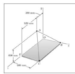
Knowing that the tension in cable AB is 1425 N, determine the components of the force exerted on the plate at B.
