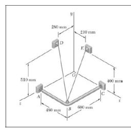
For the frame of Problem 2.87, determine the magnitude and direction of the resultant of the forces exerted by the cable at *B* knowing that the tension in the cable is 385 N.
