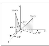
Determine (a) the x, y, and z components of the 750-N force, (b) the angles  $\theta_x$ ,  $\theta_y$ , and  $\theta_z$  that the force forms with the coordinate axes.
