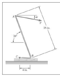
It is known that a vertical force of 200 lb is required to remove the nail at C from the board. As the nail first starts moving, determine (a) the moment about B of the force exerted on the nail, (b) the magnitude of the force  $\mathbf{P}$  that creates the same moment about B if  $a=10^{\circ}$ , (c) the smallest force  $\mathbf{P}$  that creates the same moment about B.
