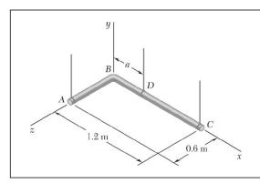
Two steel pipes AB and BC, each having a mass per unit length of 8 kg/m, are welded together at B and supported by three wires. Knowing that a = 0.4 m, determine the tension in each wire.
