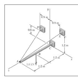
A 2.4-m boom is held by a ball-and-socket joint at C and by two cables AD and AE. Determine the tension in each cable and the reaction at C.
