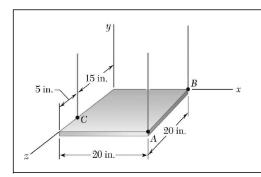
The 45-lb square plate shown is supported by three vertical wires. Determine the tension in each wire.
