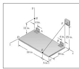
The rectangular plate shown weighs 75 lb and is held in the position shown by hinges at A and B and by cable EF. Assuming that the hinge at B does not exert any axial thrust, determine (a) the tension in the cable, (b) the reactions at A and B.
