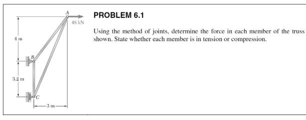
**Ans.**  $F_{AB} = 180.0 \text{ kN (T)}, F_{BC} = 144.0 \text{ kN (T)}, F_{AC} = 156.0 \text{ kN (C)}$
