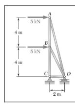
Using the method of joints, determine the force in each member of the truss shown. State whether each member is in tension or compression.
