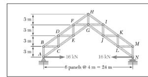
Determine the force in members DF, EF, and EG of the truss shown.
