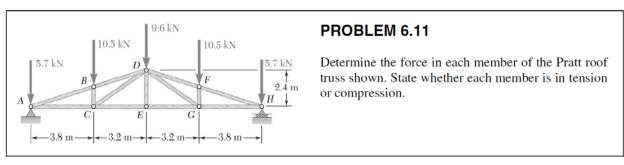
**Ans.**  $F_{AB} = 47.2 \text{ kN (C)}, F_{AC} = 44.6 \text{ kN (T)}, F_{BC} = 10.5 \text{ kN (C)}, F_{BD} = 47.2 \text{ kN (C)}, F_{CD} = 17.5 \text{ kN (T)}, F_{CE} = 30.6 \text{ kN (T)}, F_{DE} = 0.00 \text{ kN (T)}, F_{DE} =$
