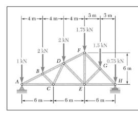
Using the method of joints, determine the force in each member of the double-pitch roof truss shown. State whether each member is in tension or compression.
