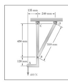
Determine the force in member BD and the components of the reaction at C.
