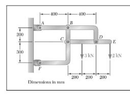
For the frame and loading shown, determine the components of all forces acting on member ABD.
