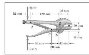
Determine the magnitude of the gripping forces produced when two 300-N forces are applied as shown.
