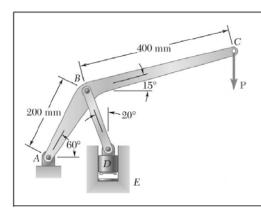
The press shown is used to emboss a small seal at E. Knowing that P = 250 N, determine (a) the vertical component of the force exerted on the seal, (b) the reaction at A.
