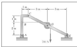
Knowing that the pulley has a radius of  $0.5\,\mathrm{m}$ , determine the components of the reactions at A and E.
