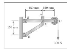
Knowing that the pulley has a radius of 50 mm, determine the components of the reactions at B and E.
