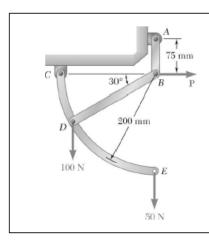
For the system and loading shown, determine (a) the force **P** required for equilibrium, (b) the corresponding force in member BD, (c) the corresponding reaction at C.
